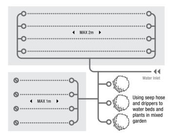
KIT REQUIRED: SOL-C24L, 12 Dripper Ext Kit, 12m Seephose Spare Capacity: 9 drippers
