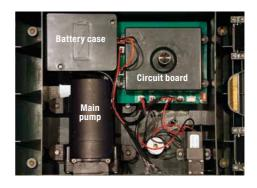
• The switch on the circuit board controls the solar panel. This is charging the battery on a 5 minute cycle. On switch positions 1,2,3,4,5, the solar panel is turned on for 1,2,3,4,5 minutes respectively. Changing the switch position will not affect the current run time or flow rate, but will control the amount of charge available for the subsequent watering cycle, thereby affecting the pumping duration. The application can be fine-tuned with small adjustments to the bypass valve.
